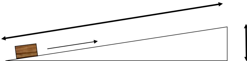
$$\text{ideal mechanical advantage} = \frac{\text{effort distance}}{\text{resistance distance}} = \frac{\text{length of ramp}}{\text{height of ramp}}$$
