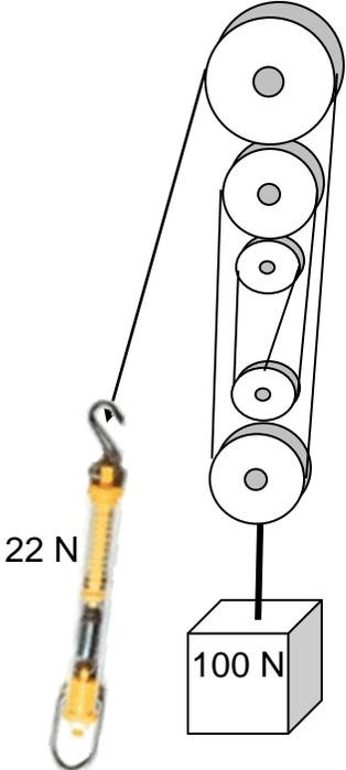
13. Determine the efficiency of the following pulley system.
