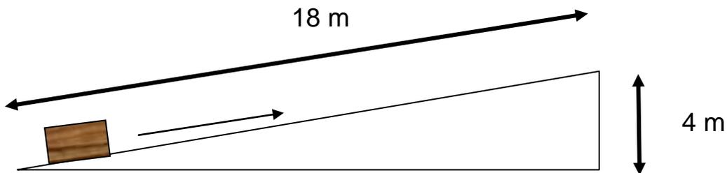
5a. To determine the AMA of the inclined plane, you must use force. The effort force is what is measured with a spring scale in Newtons. The resistance force is weight of the box in newtons.
